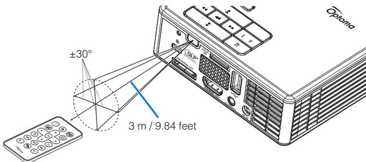
**Note:** Actual operating range may slightly differ from the diagram. Additionally, a weak battery reduces or eliminates the operating range of the remote control.
