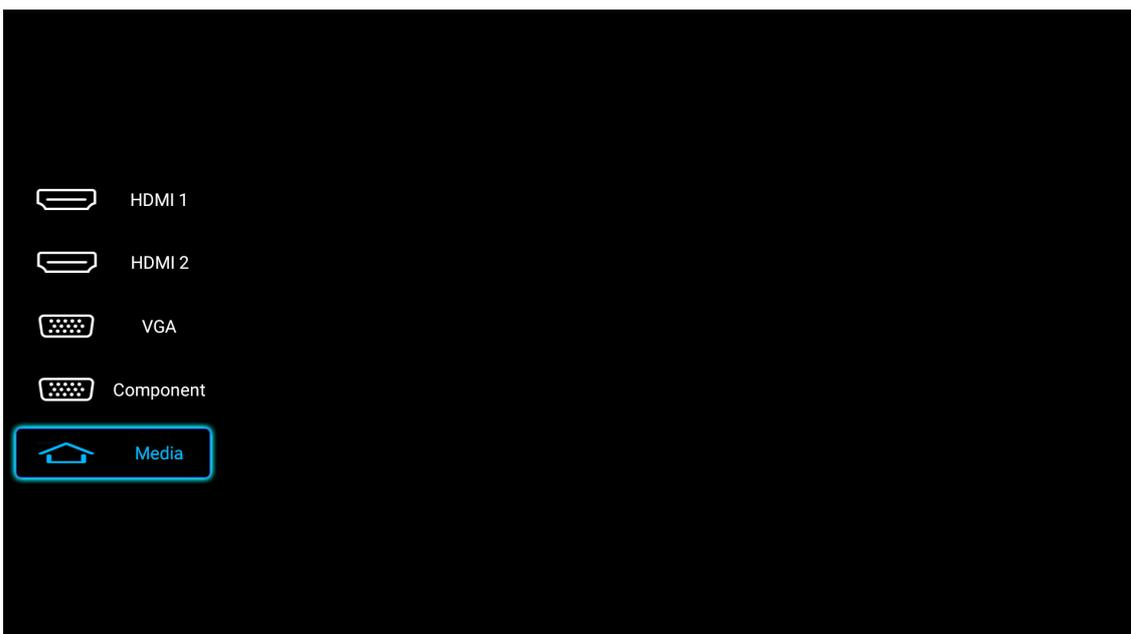
Select the desired input source and press **Enter** on the remote control or ← on the projector keypad to confirm the selection.
