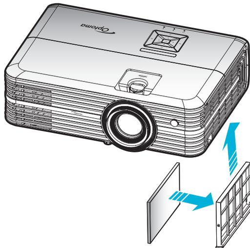
**Note:** Dust filters are only required/supplied in the selected regions with excessive dust.
