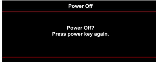
3. Press the "⏻" again to confirm, otherwise the message will disappear after a period of time (by default after 10 seconds). When you press the "⏻" button for the second time, the projector will shut down.
