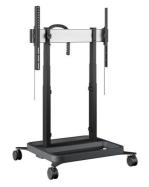
The RISE 5308 motorised display lift trolley is suitable for displays of up to 86" with a maximum weight of 120kg. The lift raises the screen smoothly, quickly, and safely at a speed of 80 mm/s with QuickRise<sup>™</sup>. With a 980mm travel range the lift is suitable for both very low and high positions.
