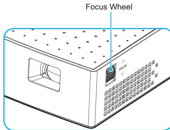
**Note:** The projector will focus at a distance of 0.6m to 1.9m.
